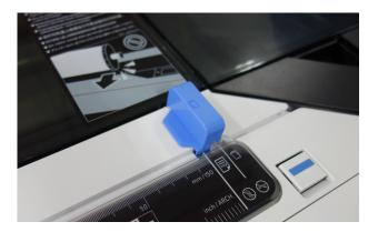
2. With the side to be scanned facing up, align the right edge of the original with the scanner edge guide.
